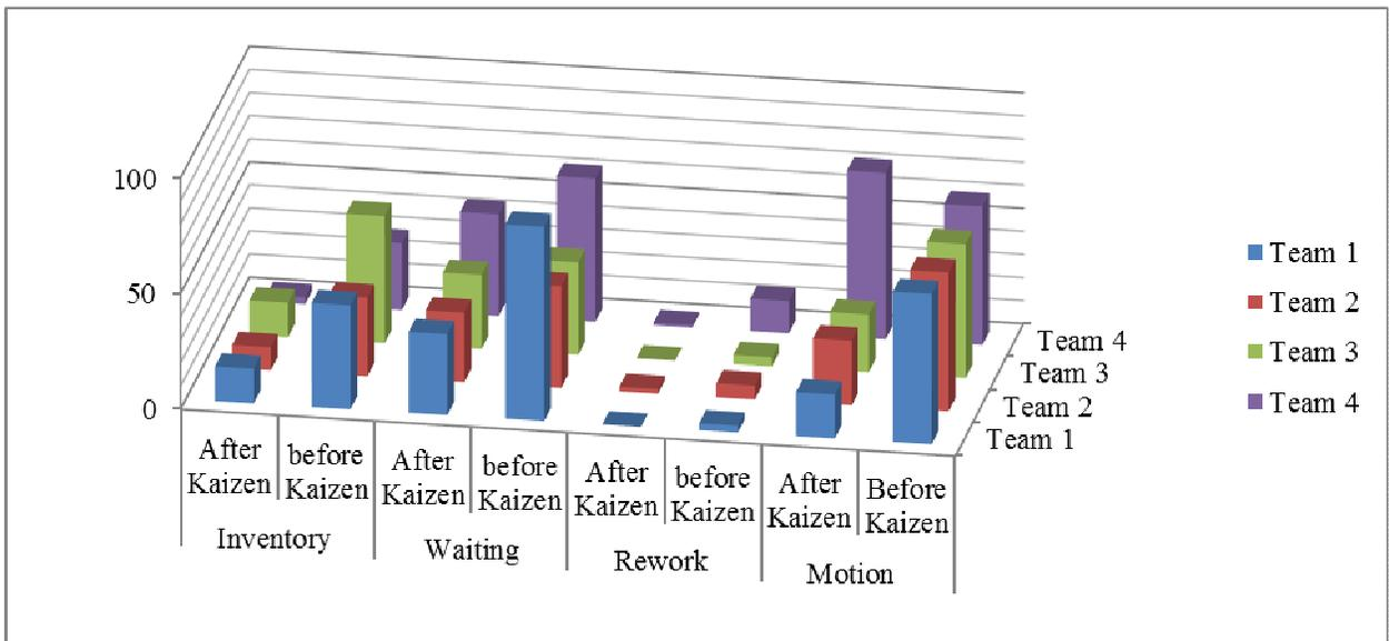
Figure 8. Before and after Kaizen mode waste identification
