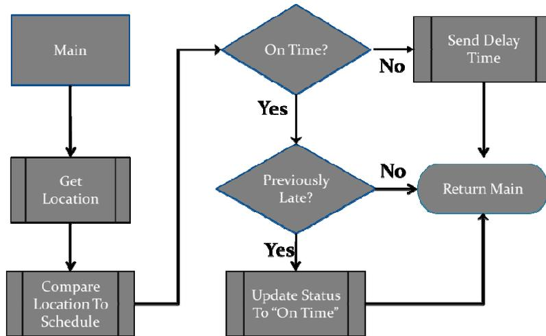
Figure 7. Bus-side application flowchart
