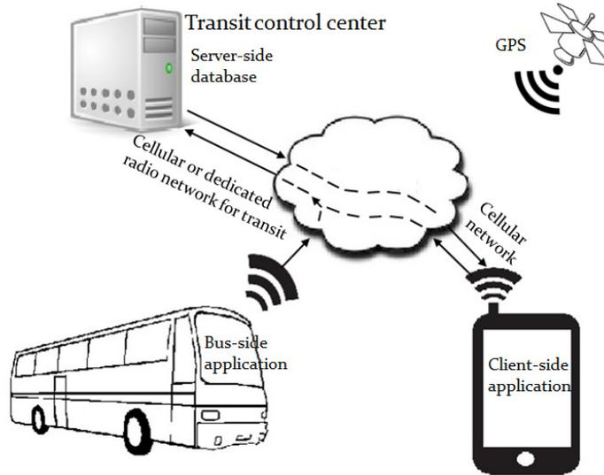
Figure 6. Bus tracking and trip planning system architecture
