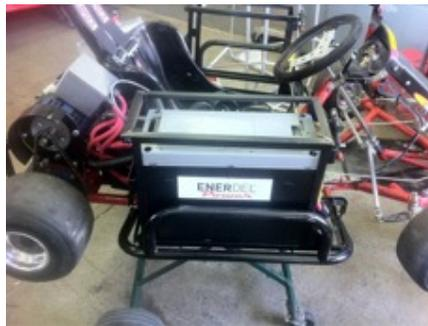
Figure 7. Student designed and built battery exchange system
