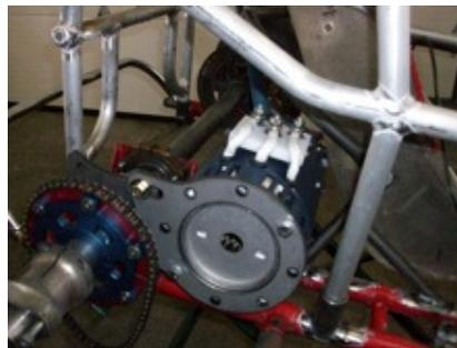
Figure 8. Student designed and built motor mounting and drive system
