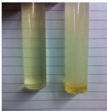
Figure 4. A passed 27/3 test using ultrasonication (left) and a failed test using conventional stirring (right)
