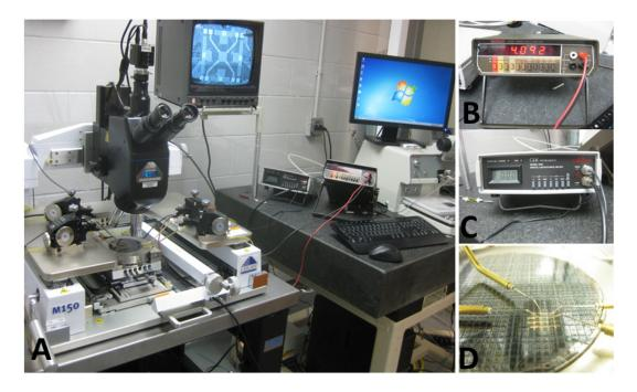
Figure 5. A) The probe and computer station where static and quasi-static tests have been performed, B) The digital multimeter, C) The capacitance meter, D) Probe tips placed on the wafer during a short test
