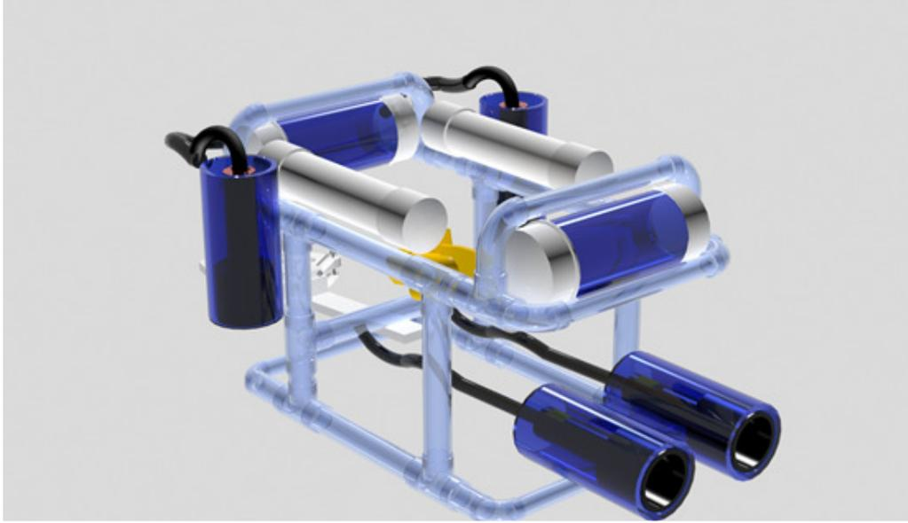
Figure 5. Partial view of the ROV model 3-D rendering
