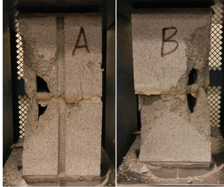
Figure 5. Example break with exposed mortar joint – adjacent faces
