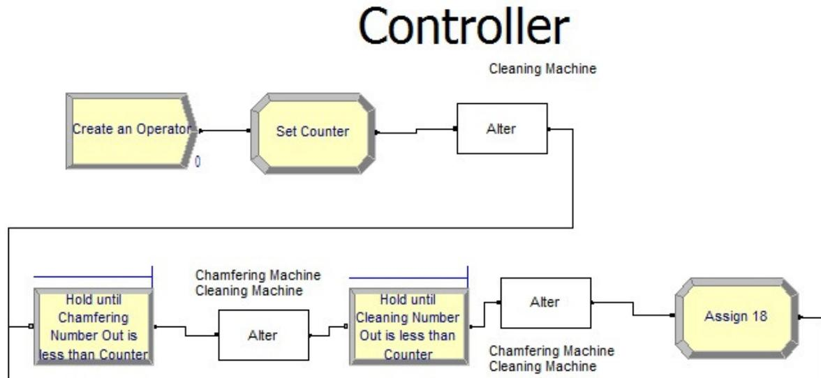
Figure 6. The controller segment (for two-operator scenario)
