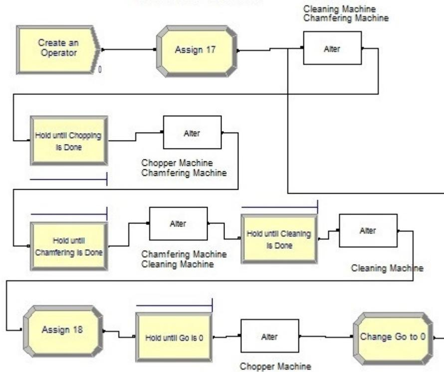
Figure 5. The controller segment (for one-operator scenario)
