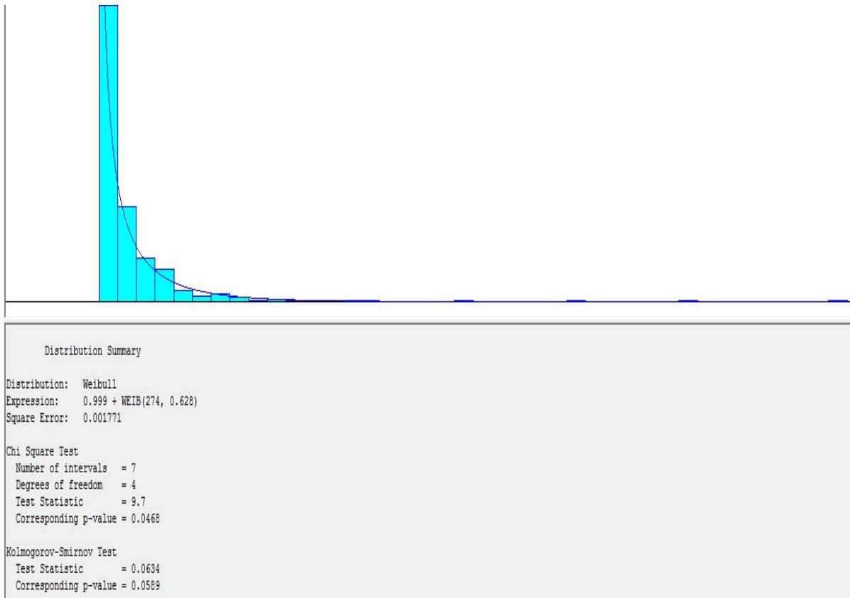
Figure 2. The probability distribution function estimated by ARENA’s input analyzer
