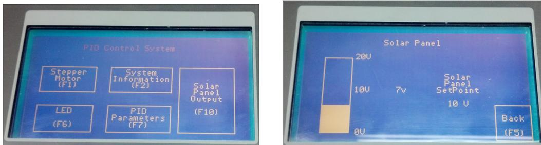
Figure 5. (a) System main menu (b) Solar panel voltage monitoring
