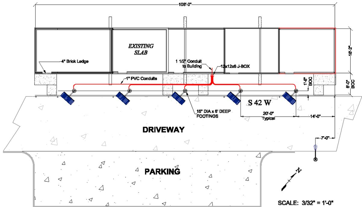
Figure 2. Layout drawing for the location of the light poles, powerhouse, and conduit
