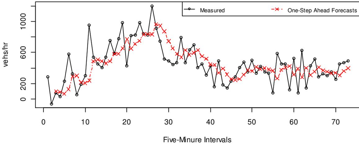
Figure 4. Eagle Road on-ramp one-step ahead flow predictions
