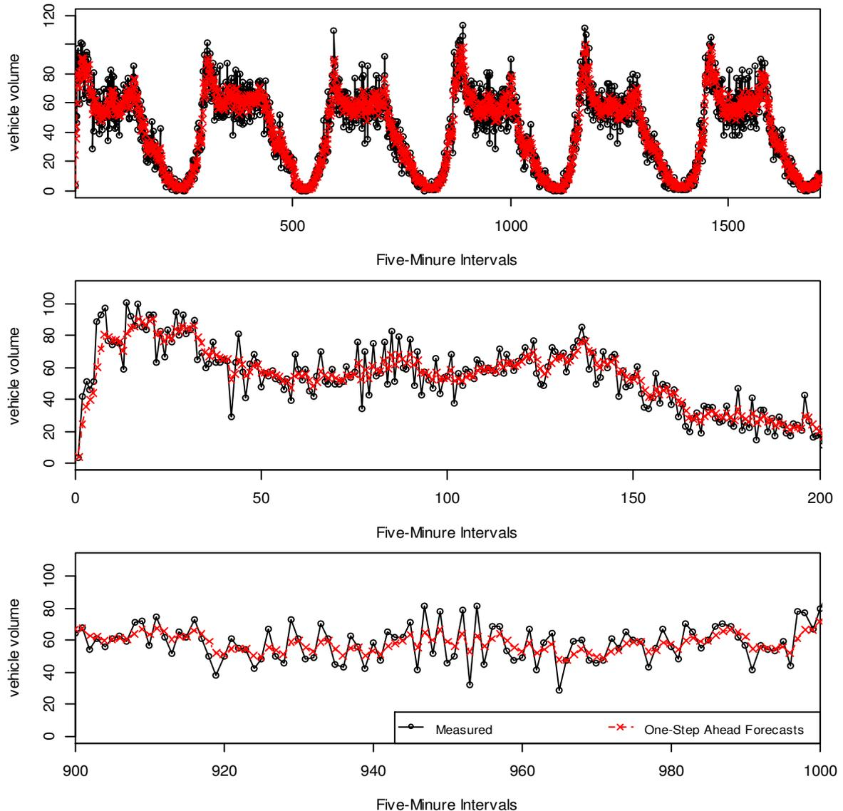
Figure 2. Measured traffic state with one-step ahead forecasts, shown in detail in second and third plots
