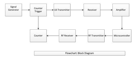
Figure 1. System block diagram
