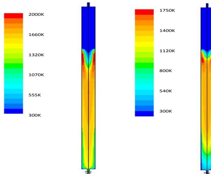
Figure 7. Contour profile of the temperature: MSW (left), oil shale (right)
