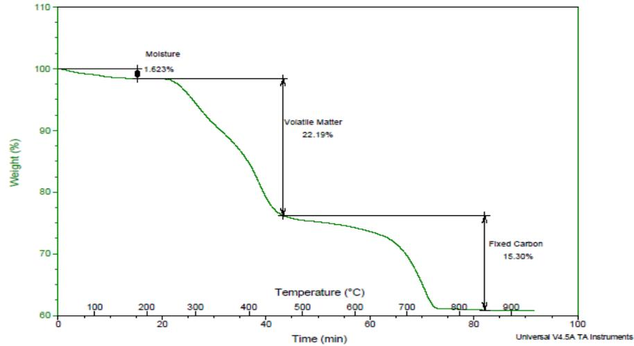
Figure 1. Proximate analysis of the El Lajjun oil shale
