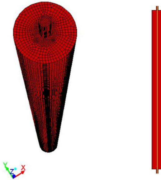
Fig. 3. The 2-D and 3-D mesh structure
