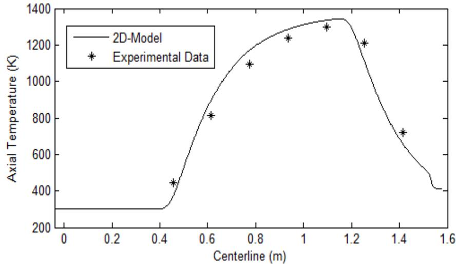
Figure 5. Axial temperature validation with experimental data for non-reactive flow
