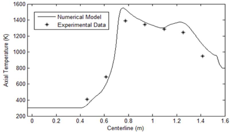
Figure 6. Axial temperature validation with experimental data for reactive flow
