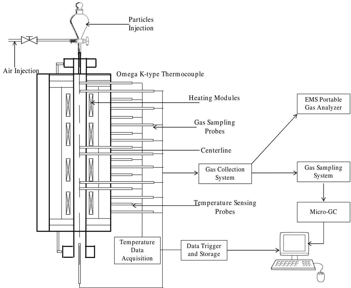
Figure 4. Schematic representation of the drop tube experimental set-up
