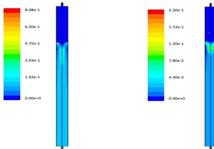
Figure 9. Contour profile of the volatile mole fraction: MSW (left), oil shale (right)
