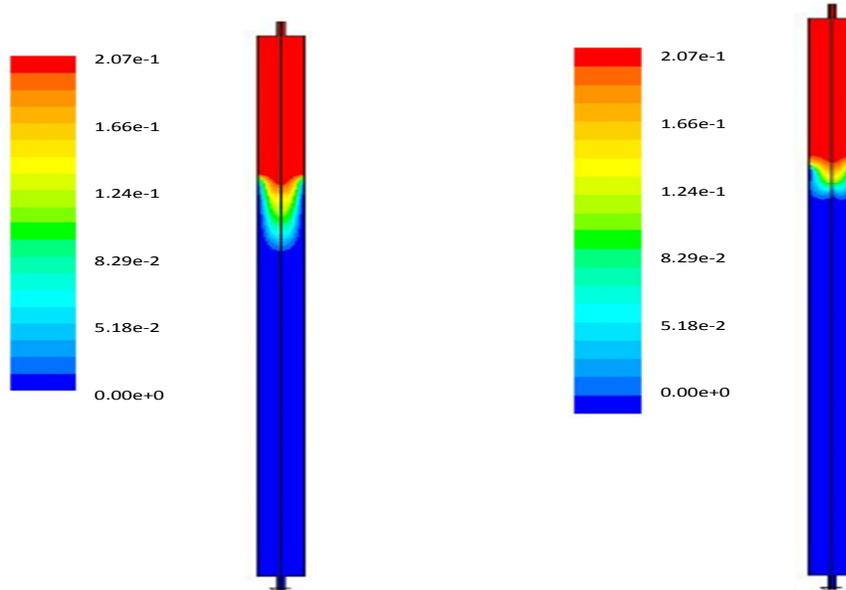
Figure 8. Contour profile of the oxygen mole fraction: MSW (left), oil shale (right)
