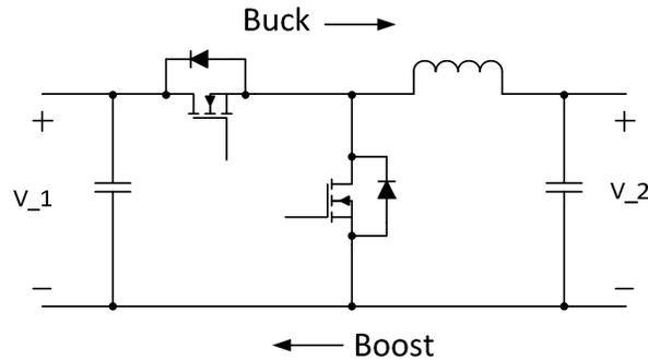
Figure 2: Bidirectional buck/boost converter.
