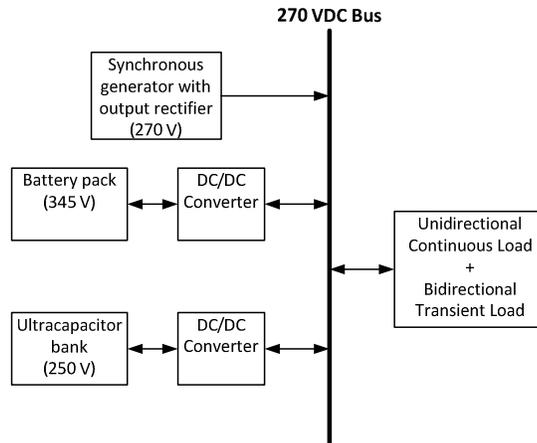
Figure 1: An example HESS system.
